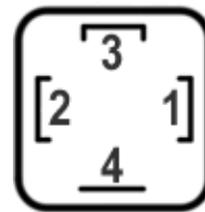
*The coil is connected between pins 1 and 2 and in the supplied harness is properly wired to the A connector of the Electronic Sensor.*
